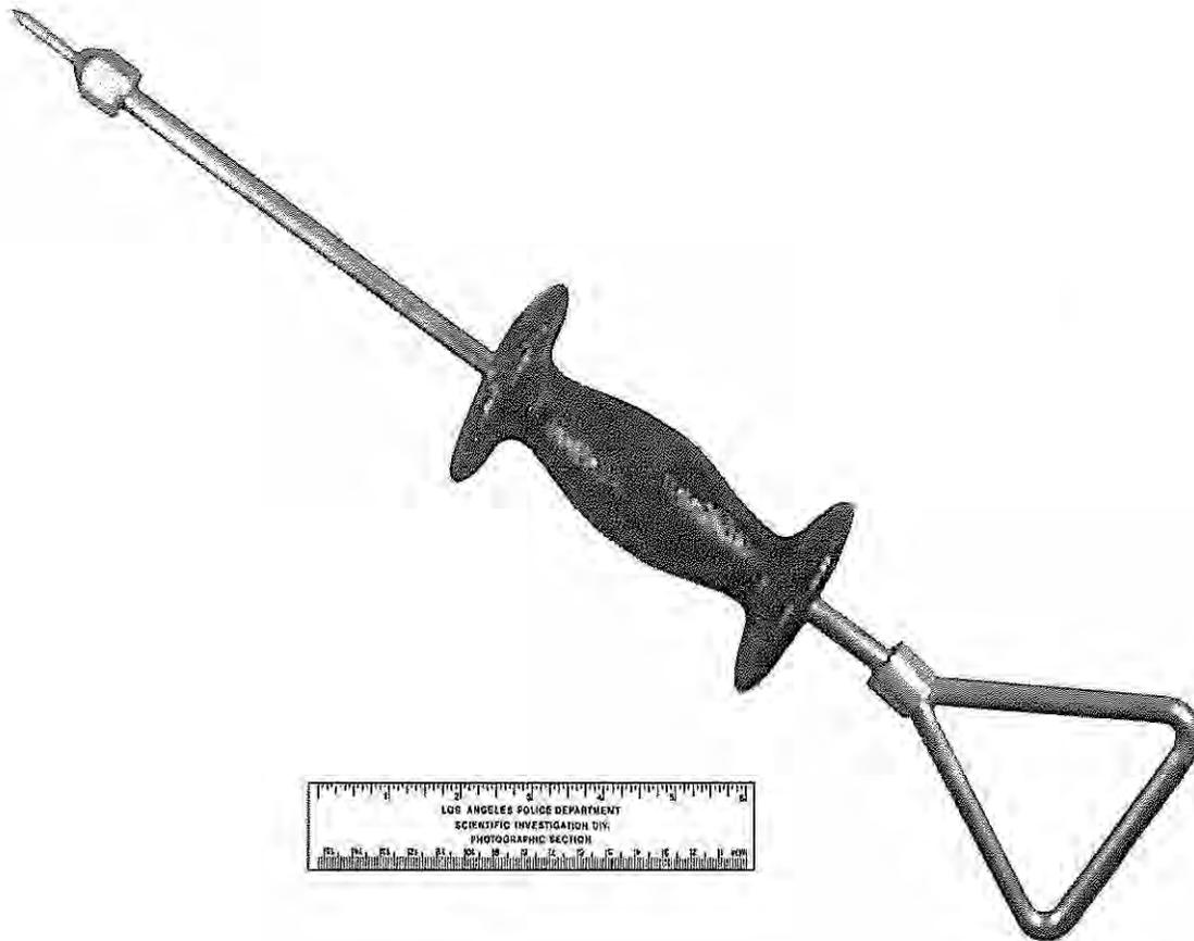
A car repair tool used to pull dents out of metal body parts, the slide hammer can be used to rip out door locks, ignition circuits, and car stereos.
